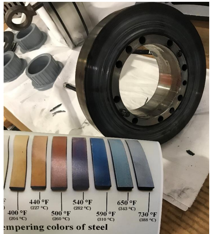
FIGURE 12: THRUST COLLAR WEAR WITH TEMPERATURE DISCOLORATION
